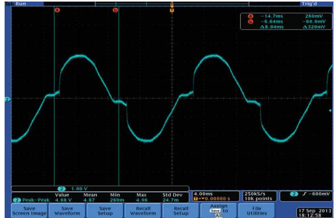
Figure 13: Plot of voltage across the terminals of the CFL with dimmer level set to 100.
