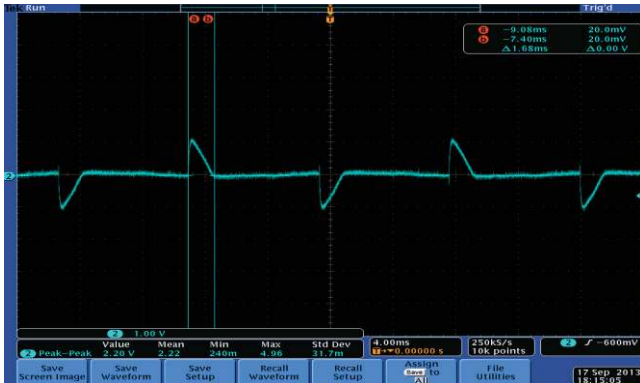
Figure 11: Plot of voltage across the terminals of the CFL with dimmer level set to 8.
