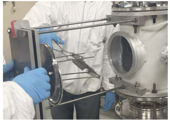
Fig. 5. Insertion of the ^7\text{Be} radioactive target in the setup, with a support independent of the telescope detector installed from the opposite side of the chamber.
