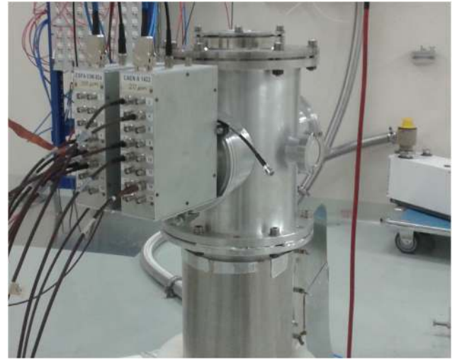
Fig. 3. The scattering chamber, with the front-end electronics, installed on the vertical neutron beam line in EAR2. The target and the telescope detector are inside.
