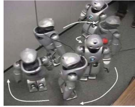
Fig. 15. Manuevering experiment using combination of CPG and state-machine controller
