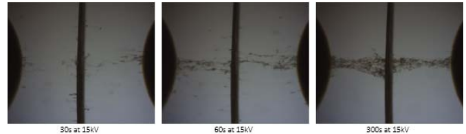
Figure 7. Optical microscopic images of bridging in contaminated transformer oil with 150-250 \mu\text{m} pressboard fiber and Kraft paper barrier, concentration level 0.001%.
