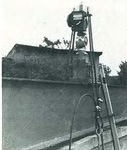
Fig. 15a. Closeup of recording dynamometer on test girder.
