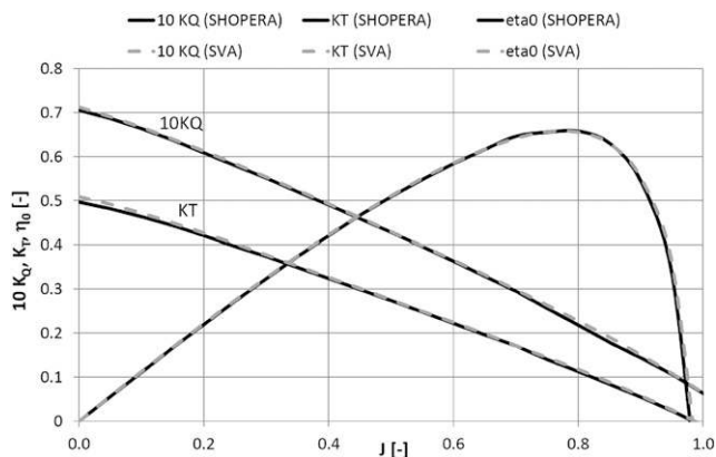
Fig. 20 Model scale open water diagram for the DTC propeller comparing data measured at MARINTEK (scale 1:63.65) and SVA Potsdam (scale 1:59.406, see El Moctar et al. 2012)
