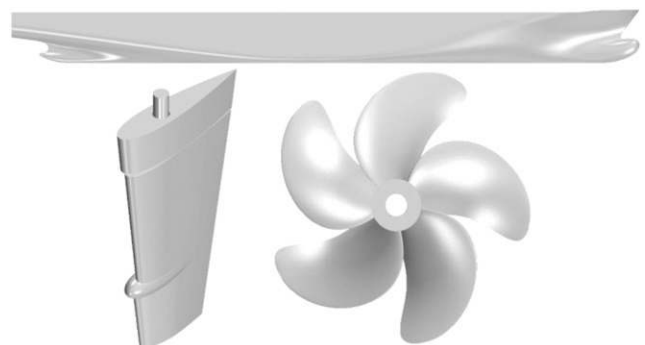
Fig. 2 View of the DTC hull (top), the rudder (bottom, left) and the propeller (bottom, right)
