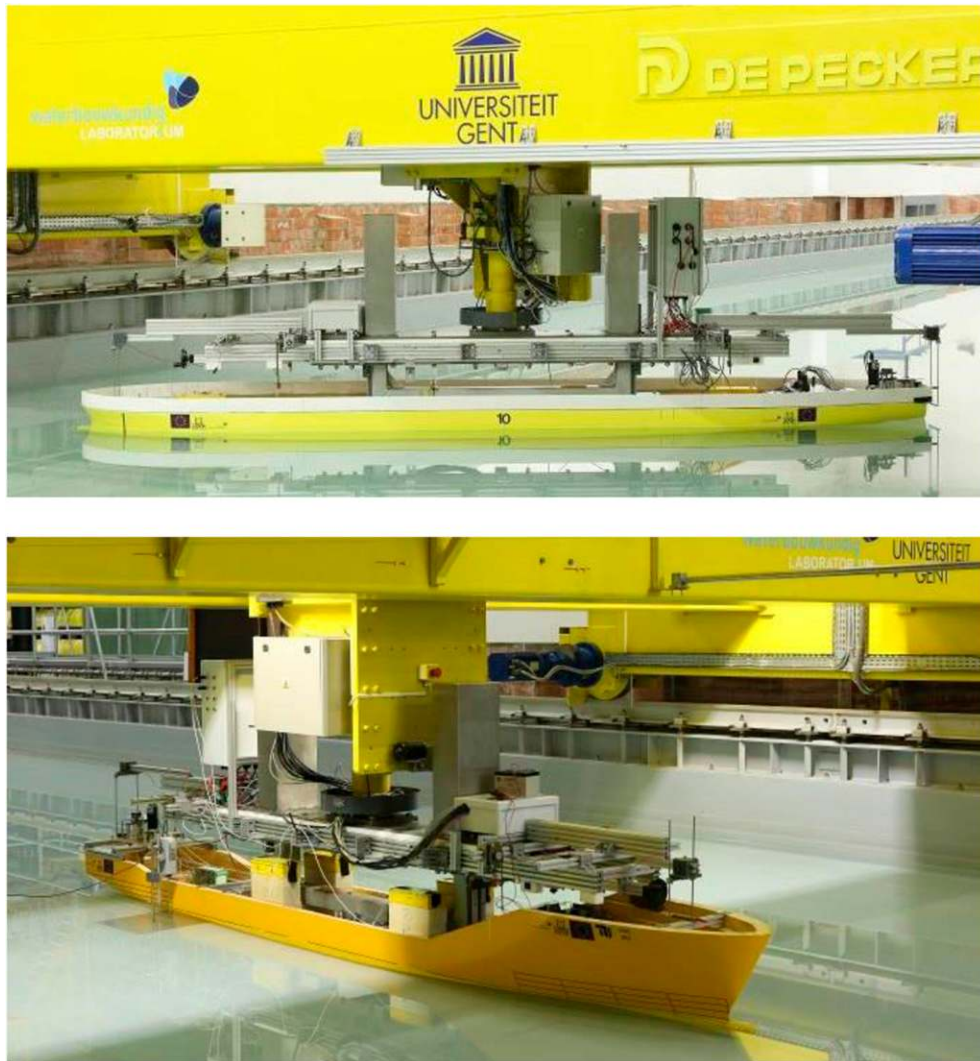
Fig. 5 Impressions of the KVLCC2 (top) and DTC model (bottom) in the captive test setup at FHR
