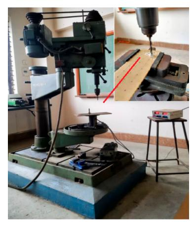
Figure 3. Actual setup of drilling operation with dynamometer.
