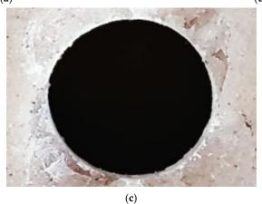
**Figure 16.** Hole quality assessment using light microscopy. (**a**) A 6 mm diameter drill, (**b**) 8 mm diameter drill, (**c**) 10 mm diameter drill.
