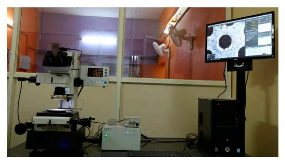
Figure 5. Light microscope used for hole quality assessment.
