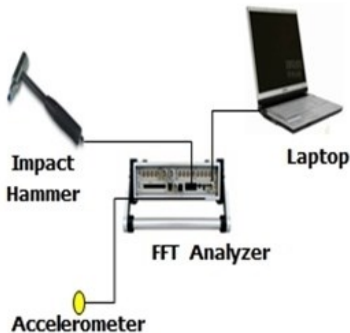
Figure 40 – Setup for the Experimental Modal Analysis
