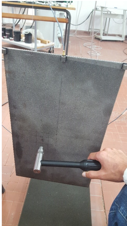
Figure 41 – Final test setup with suspended elastic connections of plate specimen
