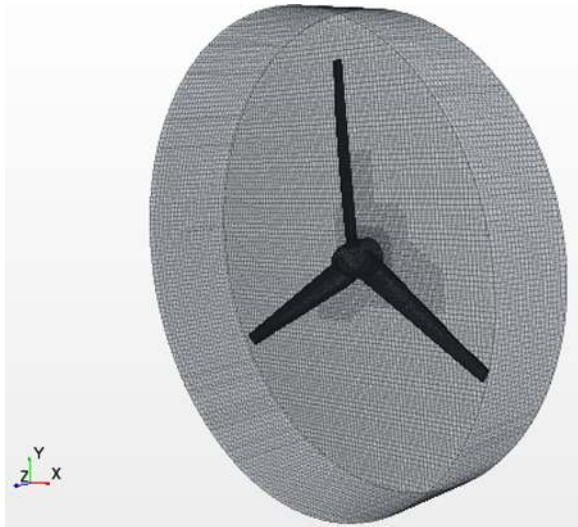
Fig. 31 Rotating subdomain using trimmed mesh model with prism layer meshing at rotor surfaces
