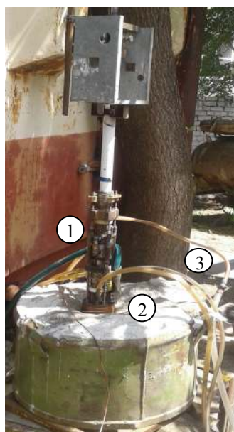
Fig. 1. Experimental set up for the study of the borehole thermal reaming process in the granite block by means of angular plasmatron: 1- plasmatron; 2- granite block; 3- cooling system of the plasmatron.
