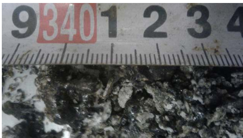
Fig. 3. Spalls of rock after the thermal reaming of the borehole by means of the angular plasmatron.
