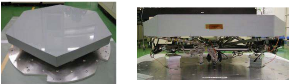
Figure 9. The segmented mirror Sub-ASSY after polishing. (left): Appearance of after polishing (the configuration of the surface figure measurement). (right): side view with the 6-axes adjustment mechanisms and the curvature adjustment mechanisms after Sub-ASSY integration #2.
