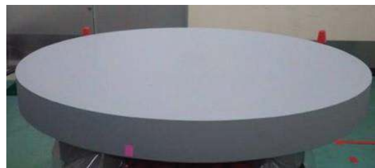
Figure 6. Appearance of the segmented mirror at the stage of “circular shape processing”. (left): stage prior to ceramic sintering (after lightweight processing). (right): stage when the “circular shape processing” was completed.
