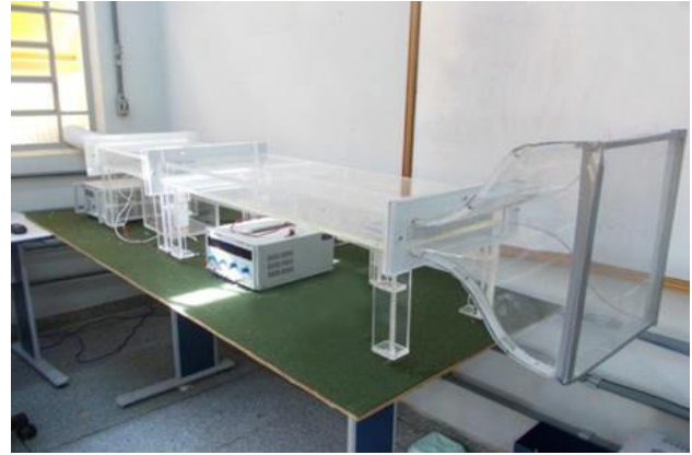
(a) Suction type wind tunnel with open return
