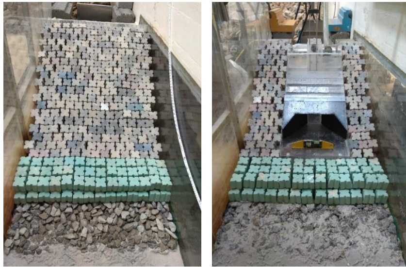
Figure 8. Physical model without (left) and with (right) the hybrid WEC module (geometry B) integrated in the breakwater and before the experimental tests.
