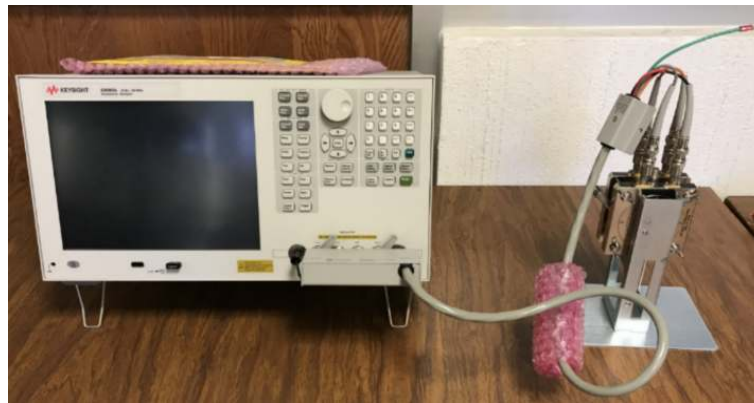
Figure 6. Experimental array for measurements of electrical impedance of commercial drugs. Impedance analyser and Liquid Test Fixture schematic.
