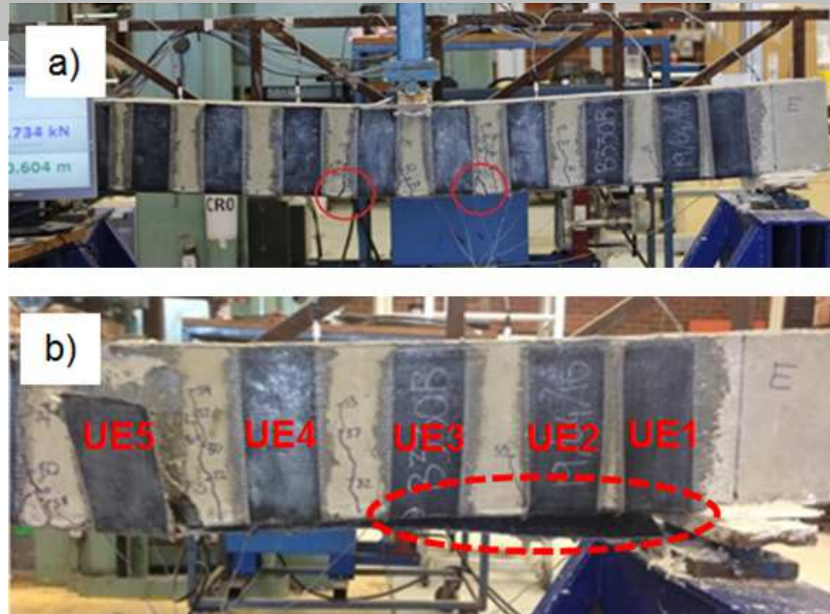
Figure 18 (a) Intermediate crack induced interfacial debonding of soffit strip of B330B; (b) Complete failure of B330B by debonding of soffit strip and rupture of UE1, UE2 and UE3
