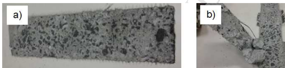
Figure 16 (a) Interfacial failure of the soffit strip, (b) Concrete cover separation of the U-jacket
