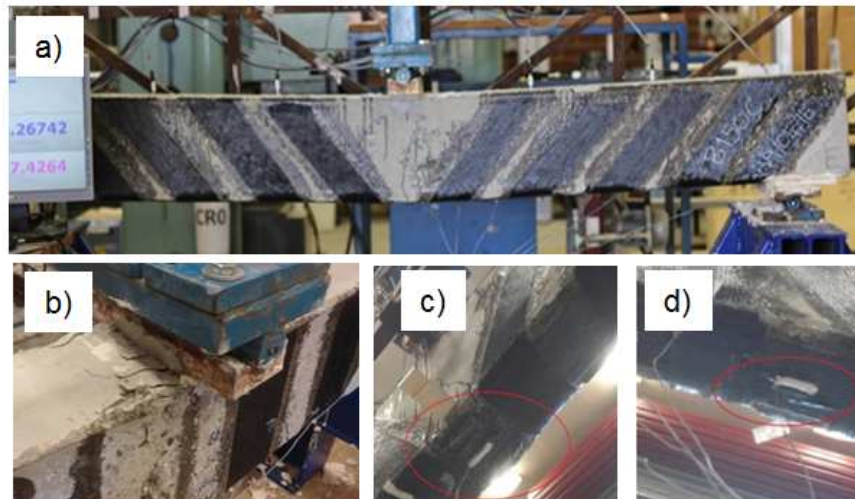
Figure 13 (a) Failure mode of Beam B150C; (b) Compressive failure of concrete at loading plate; (c) Complete BFRP rupture at mid-span; (d) Partial BFRP rupture at SGE3
