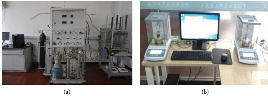
FIGURE 5: Experimental apparatus: (a) modified conductivity apparatus and (b) spontaneous imbibition device.
