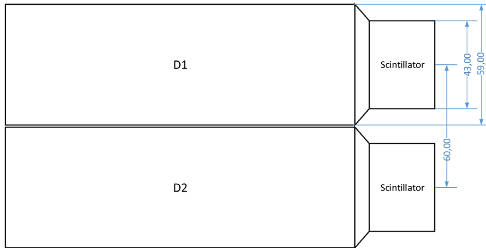
Figure 5. How the two cylindrical LaBr 3 scintillation detectors are placed next to each other. The detectors register an x-ray signal simultaneously during some discharges. This proves that the photon flux is high enough to cause a multiphoton registration at one detector.
