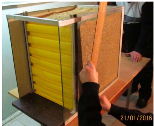
Fig. 4. Experimental capacity with the square profile with smaller plate oriented to bulk material under full load
