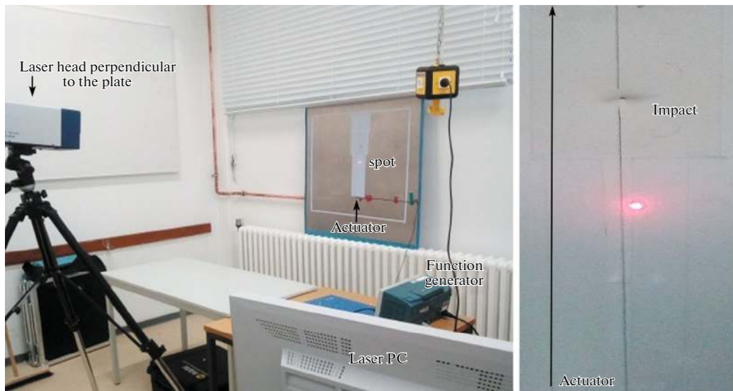
Fig. 4. (a) LDV experimental setup, (b) the scanned line for the LDV.
