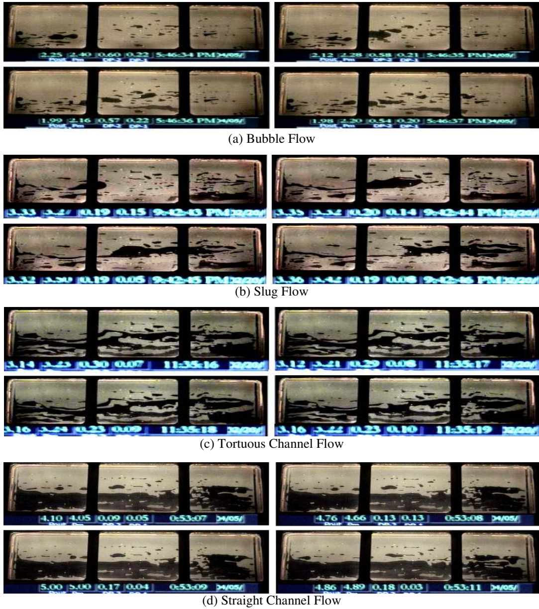
Figure 8. Photographs of flow structures in the smooth-walled fracture. Each set contains four continuous images. Flow direction was from left to right.
