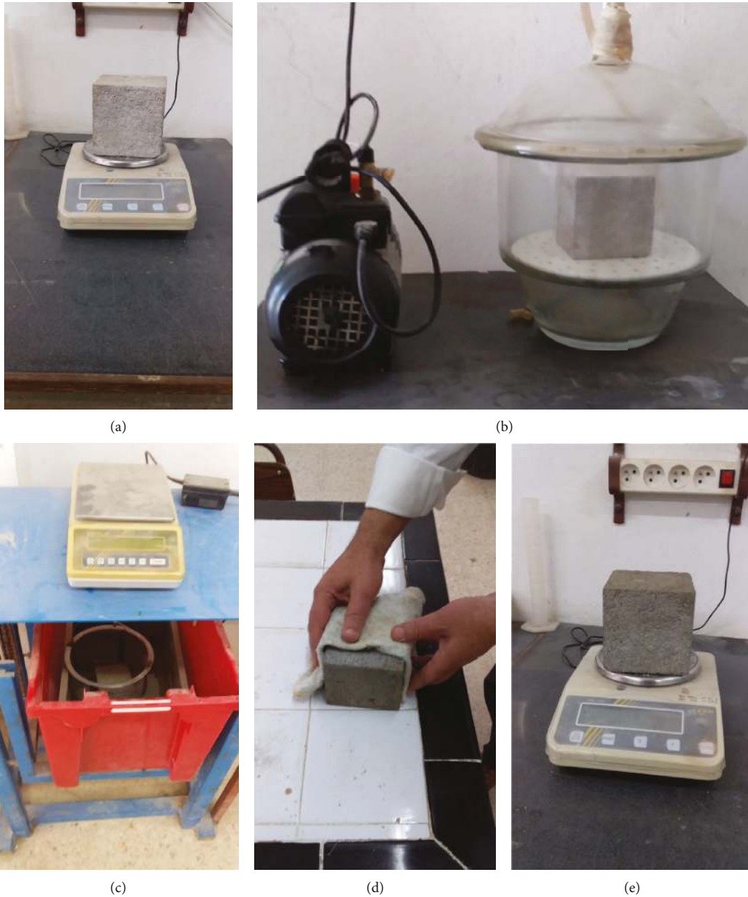
FIGURE 5: Steps of the porosity measurement test.
