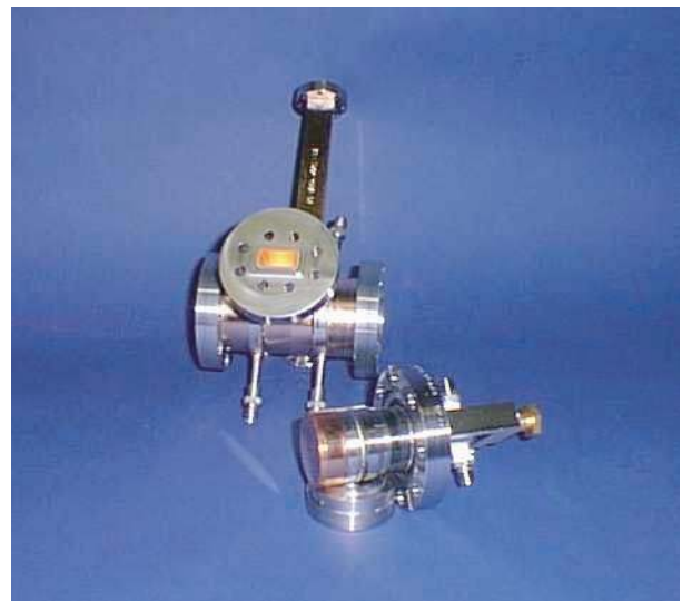
FIG. 4. (Color) A picture of the cavity body with one end cap shown on the outside. The water-cooling pipes can be seen on the bottom of the cavity body.
