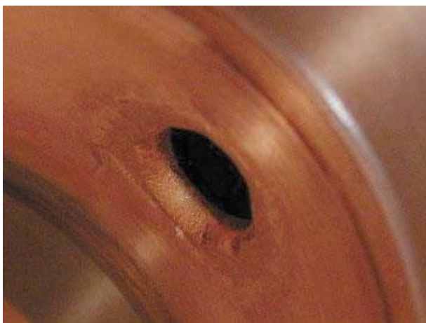
FIG. 22. (Color) A picture of the high-power coupling aperture of cavity 1 after the first high-power test. The aperture has been rounded in the direction of the magnetic field. The electric field has caused pitting to occur on either side of the aperture at right angles to the rounding.
