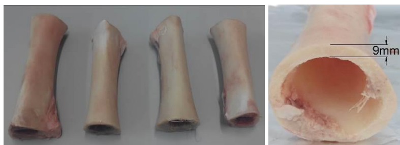
Fig. 2 - Ex-vivo bone specimens cut from middle diaphysis
