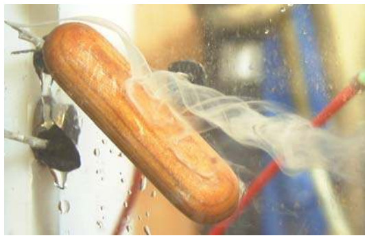
Figure 3: Vortex visualization by dye injection, for Re=1000 , behind a generator of the first column.
