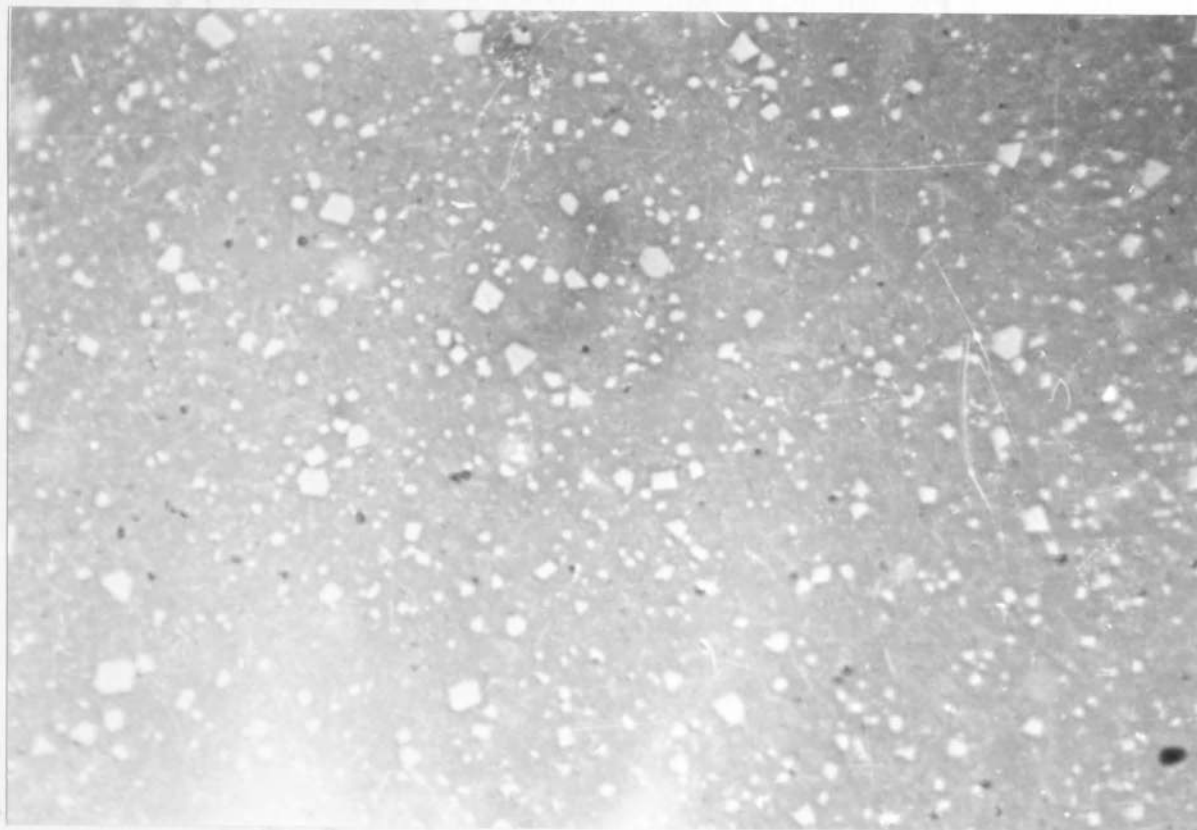
Fig. 4.10. Euhedral spinel (high relief) at 1100^{\circ}\text{C} , 9 kb (run 1995); polished mount, 650X.
