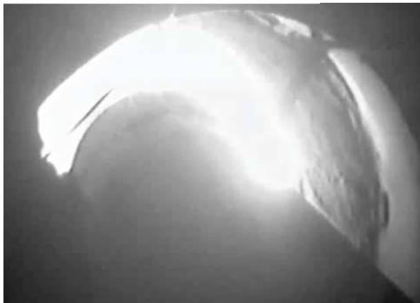
Fig. 9. Coal dust ignited in 10 min. after the plasmatron was switched on supplies to the boiler for time range \tau=12-14 min.
