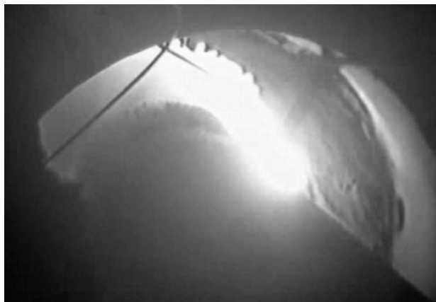
Fig. 8. Unignited coal dust supplies to the boiler when plasmatron is switched off for time range \tau=0-2 min.
