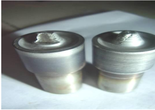
Figure2. Tools used in Friction Stir Welding (Half grooved tool & taper threaded tool)
