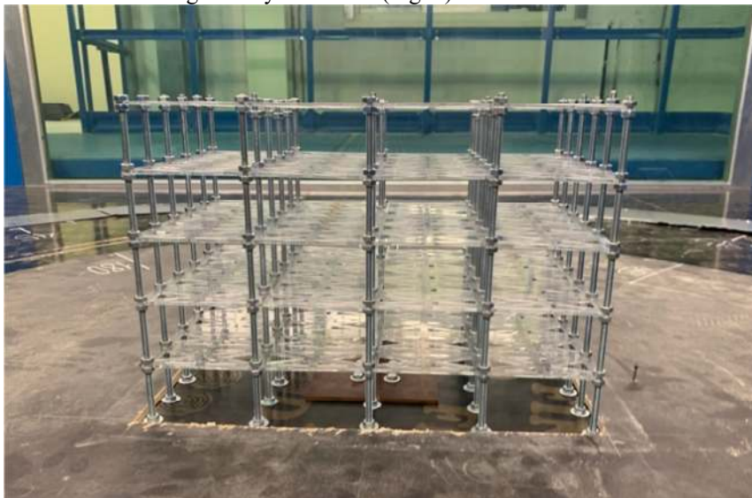
Fig. 4. Industrial scaffolding dummy. Side view.
