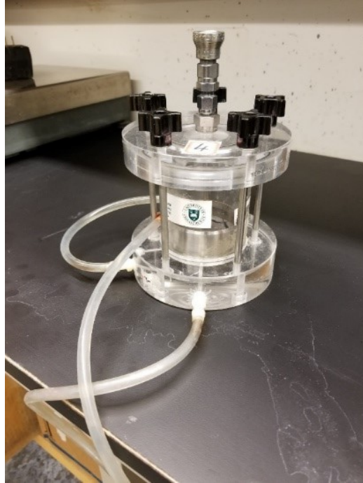
Figure 4. 3 U of S Pressure plate cell for SWCC test on suction ranges 0 to 400 kPa.
