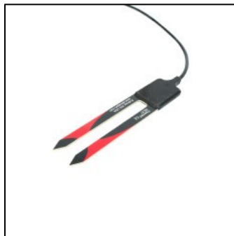
Figure 4. 21 Volumetric water content measuring sensor from Meter©.
