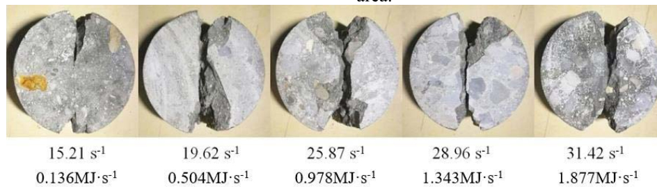
Figure 6. Typical failure mode of PC group specimens.
