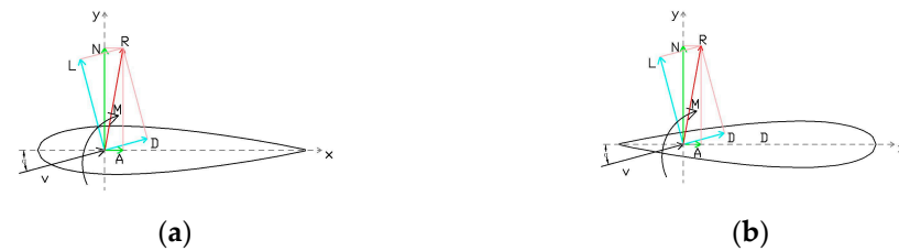
Figure 8. Definition of lift coefficient and moment coefficient in positive and negative directions. (a) Forward-blowing, (b) reverse blowing.
