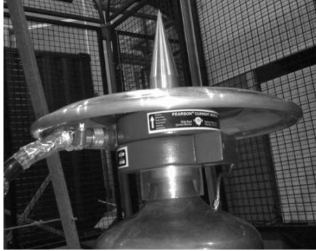
Figure 5.5: Photograph of set-up for testing the current waveform measured directly (upper probe) and the current waveform obtained through the optical fiber data transmission system (lower probe).
