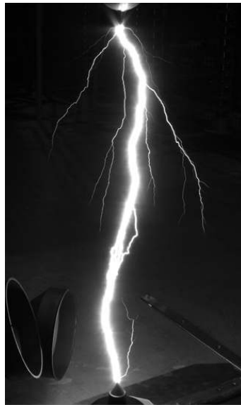
Figure 5.8: A still photograph of a positive polarity spark discharge (please ignore the reflections on the two tubes).
