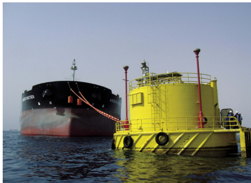
Figure 1. CALM buoy with two hawsers attached to the FPSO for loading and offloading operations (reproduced, with permission, courtesy: Bluewater; Source: Bluewater, [69]).
