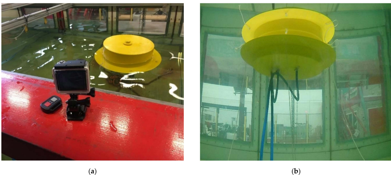
Figure 10. Setting up the CALM buoy model, showing (a) the underwater camera and top view of the buoy, and (b) underwater view of the buoy and submarine hoses (with reflection of buoy's skirt).
