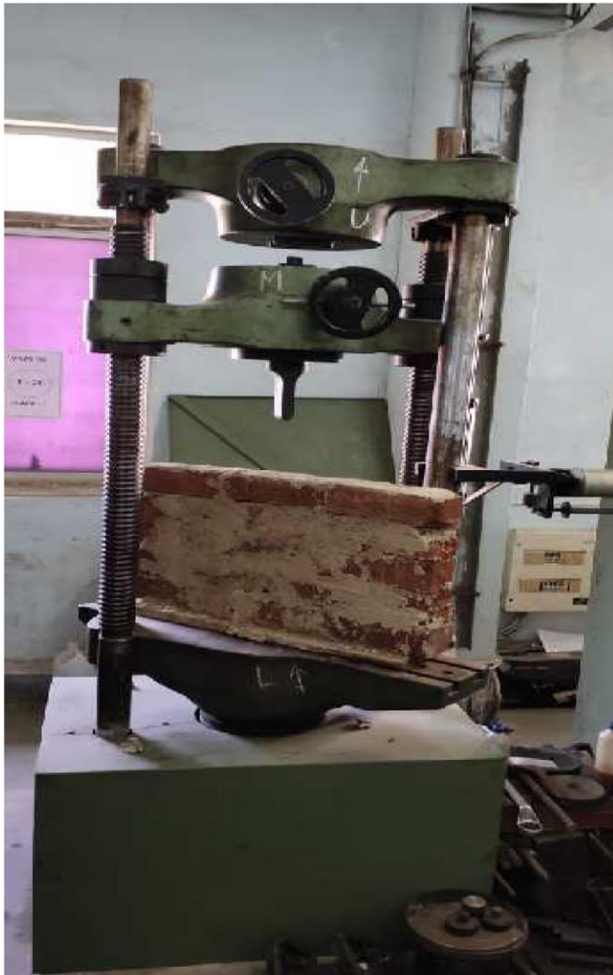
Fig. 1: First Crack Experimental Setup
