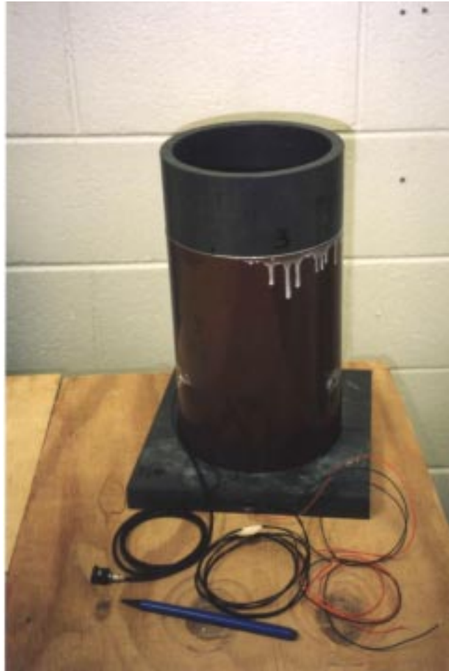
Figure 4.27 PVC “extenders” used during pluviation of samples.
