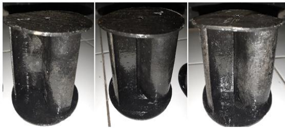
Figure 5. Rotors Variation (a) Blade arc angle120° (b) Blade arc angle135° (c) Blade arc angle150°
