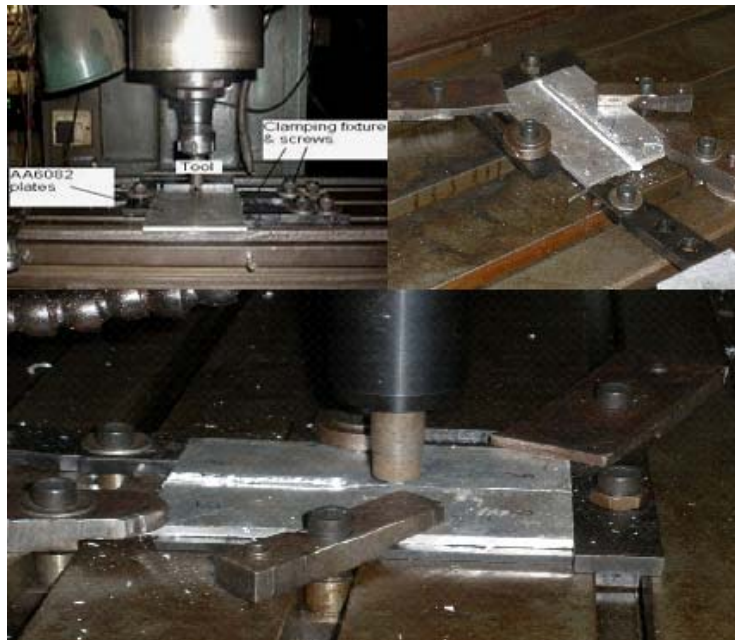
Figure 3 Experimental Setup describing clamping and welding of FSW plates
