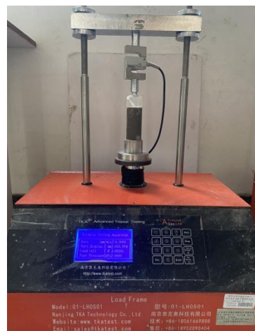
Figure 5. Fully automatic multi-functional unconfined compression instrument.
