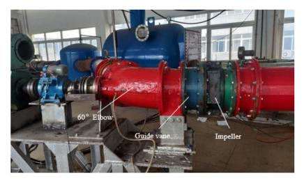
Figure 4. Schematic diagram of the experimental pump section after installation and splicing.
