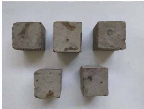
Figure 18. Evidence of sample frosting.
