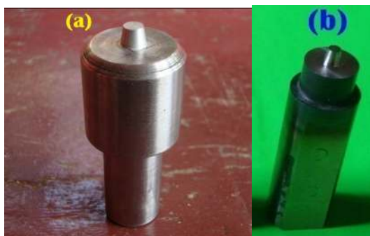
Figure 2. Photographs of the different designs of the FSW tools employed in this investigation (a) stepless cylindrical shoulder tool shoulder and (b) stepped tool shoulder
