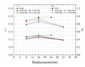
**Figure 14.** Curves of the energy-dissipation coefficients and damping coefficients at characteristic points of each specimen.
