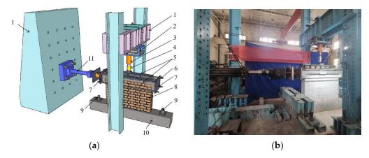
**Figure 5.** Test setup and instrumentation. (a) Schematic of the test setup: 1. Reaction wall; 2. Sliding roller; 3. Vertical jacks; 4. Vertical force sensor; 5. Distribution beam; 6. Tie rod; 7. Splint; 8. Wall; 9. Ground anchor bolts; 10. Floor beams; 11. MTS. (b) Test site.
