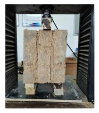
Figure 4. Shear-strength test of masonry.
