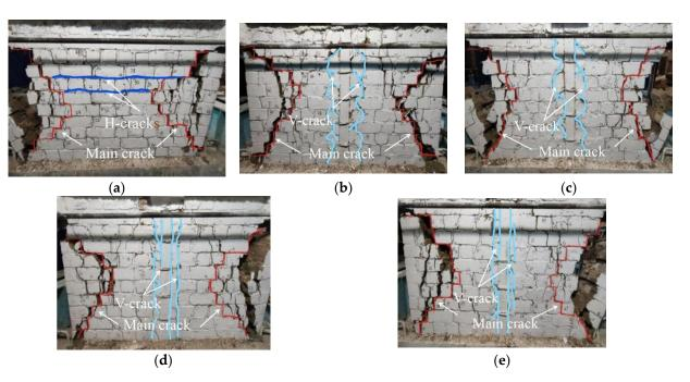
**Figure 8.** Collapse failure modes of specimens: (**a**) EAW, (**b**) EAW–MS, (**c**) UAW–MS, (**d**) EAW–MN, and (**e**) UAW–MN.
