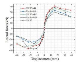
Figure 10. Skeleton curve of each specimen.
