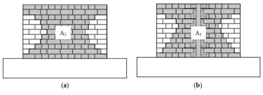
Figure 12. Schematic diagram of wall residual-area calculation: (a) adobe wall and (b) composite wall.
