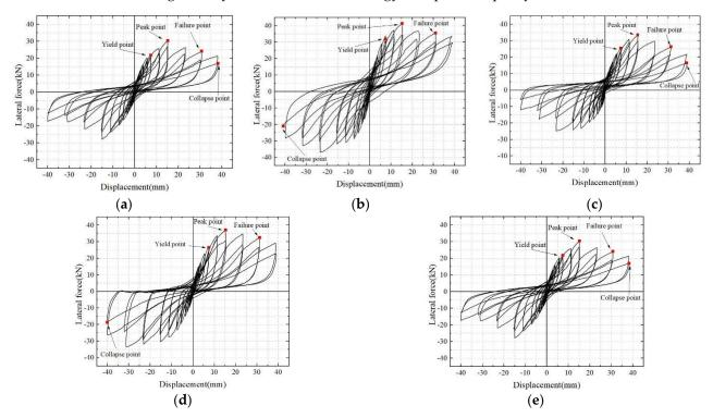
**Figure 9.** Hysteretic curve of each specimen: (**a**) EAW, (**b**) EAW–MS, (**c**) UAW–MS, (**d**) EAW–MN, and (**e**) UAW–MN.
