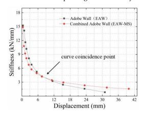
Figure 15. Composite-wall and adobe-wall stiffness degradation curves.
