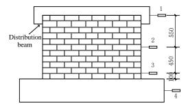
Figure 7. Layout of displacement gauge.
