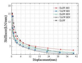
Figure 11. Stiffness degradation curve of each specimen.
