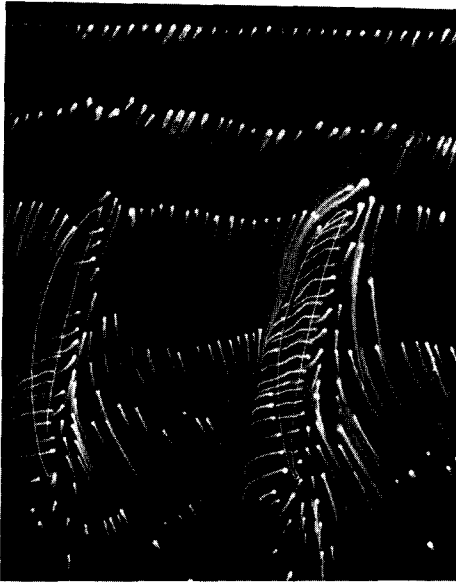
Fig.3 Paint-trace visualization on the endwall, at 2.0% tip clearance
