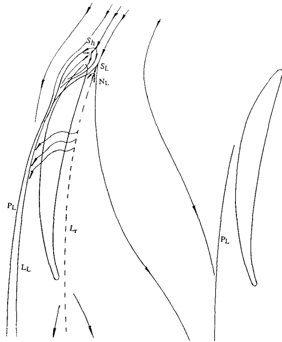
Fig.5 Schematic of the flow pattern on the wall at \tau/c=0.02
