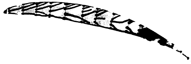
Fig.4 Ink-trace visualization on the blade tip surface, at 2.0% tip clearance
