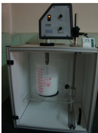
Figure 1. The nanofluid in UP 400s ultrasonic processor
