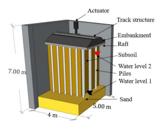
Figure 1. Geometric structure layout of track structure and piled raft foundation.
