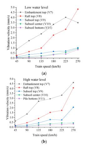
**Figure 17.** Relationship between vibration velocities and train speed at V7 to V11. (**a**) low water level (**b**) high water level.
