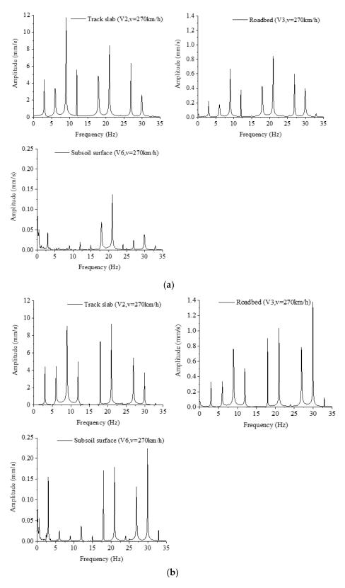
**Figure 8.** Frequency contents of velocity at track V2, V3, V6. (a) Low water level, v = 270 km/h, (b) High water level, v = 270 km/h.
