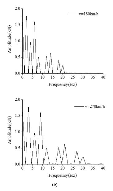
**Figure 4.** Loading curves at reduced scale for train speed of 180 km/h and 270 km/h in time and frequency domain. (**a**) time domain; (**b**) frequency domain.
