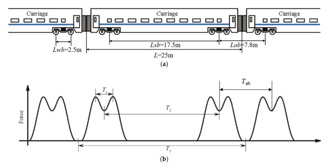
**Figure 3.** Geometry configuration of the high-speed trains and M-shaped wave. (**a**) Geometry configuration of the high-speed trains; (**b**) M-shaped wave.
