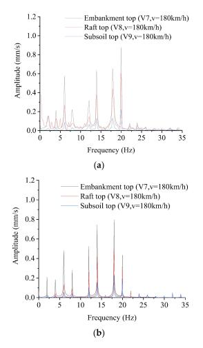
**Figure 11.** Frequency contents of vibration velocities at embankment top V7, raft top V8, and subsoil top V9. (**a**) Low water level, (**b**) High water level, v = 180 km/h.
