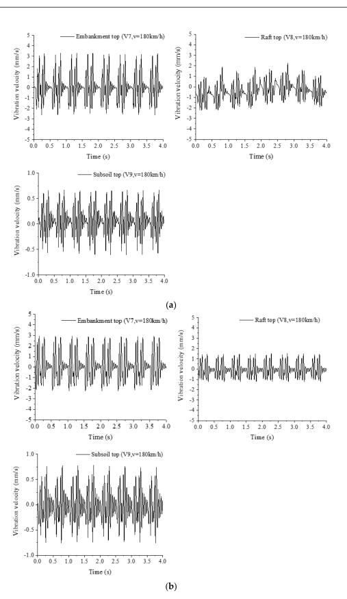
**Figure 9.** Time histories of vibration velocities at embankment top V7, raft top V8, and subsoil top V9. (a) Low water level v = 180 km/h, (b) High water level, v = 180 km/h.
