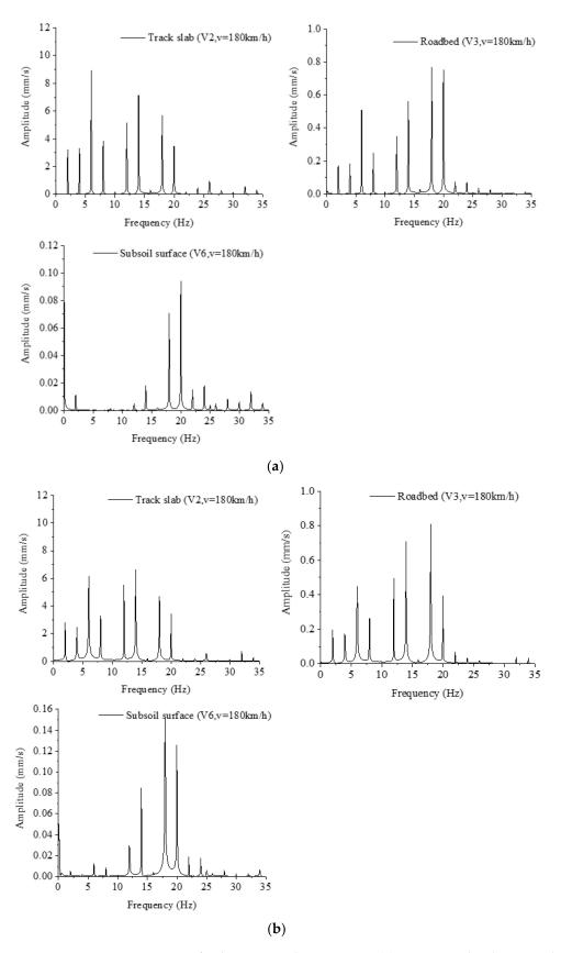
**Figure 7.** Frequency contents of velocity at track V2, V3, V6. (a) Low water level, v = 180 km/h, (b) High water level, v = 180 km/h.
