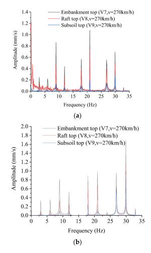
**Figure 12.** Frequency contents of vibration velocities at embankment top V7, raft top V8, and subsoil top V9. (a) Low water level, (b) High water level, v = 270 km/h.
