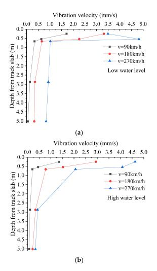
**Figure 15.** Vibration velocity distribution in vertical direction along the depth from roadbed. (**a**) low water level, (**b**) high water level.
