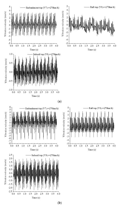
**Figure 10.** Time histories of vibration velocities at embankment top V7, raft top V8, and subsoil top V9. (a) Low water level v = 270 km/h, (b) High water level, v = 270 km/h.
