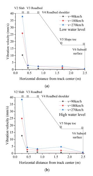
**Figure 13.** Vibration velocity distribution in horizontal direction from the track center. (**a**) low water level, (**b**) high water level.
