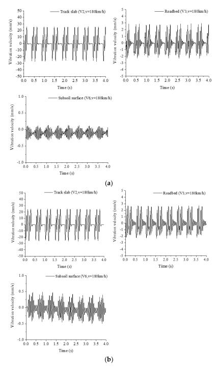
**Figure 5.** Time histories of vibration velocity at track slab V2, roadbed V3, and subsoil surface V6. (a) Low water level v = 180 km/h, (b) High water level, v = 180 km/h.
