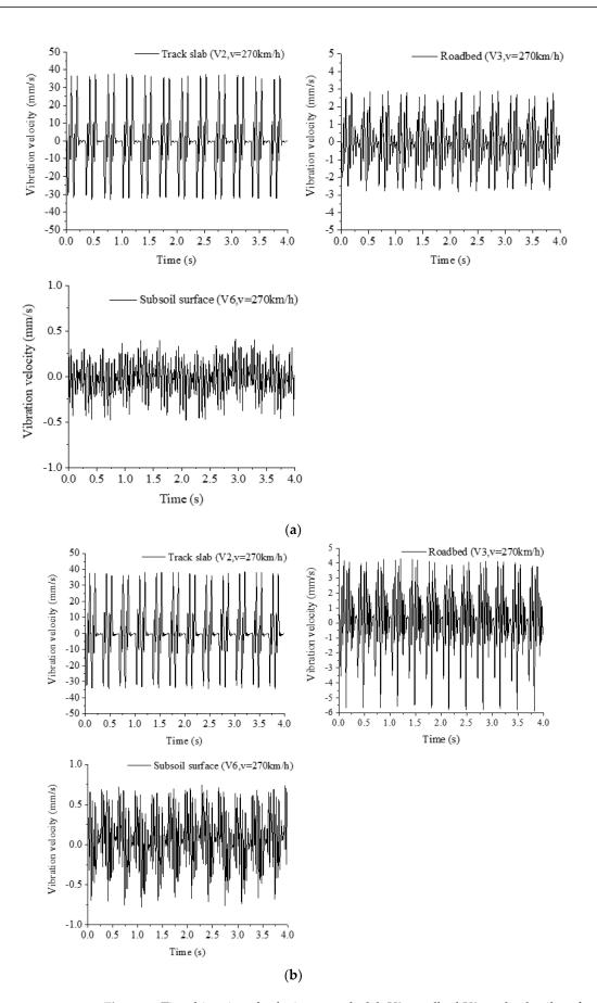
**Figure 6.** Time histories of velocity at track slab V2, roadbed V3, and subsoil surface V6. (a) Low water level, v = 270 km/h, (b) High water level, v = 270 km/h.
