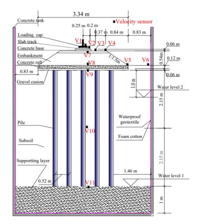
Figure 2. Layout of experimental model.
