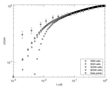
**Figure 6.** Comparison of the normalized velocity profile for different mesh resolution plotted in log-log scale.
