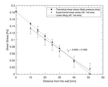
Figure 3. Theoretical and experimental shear stress across the pipe.
