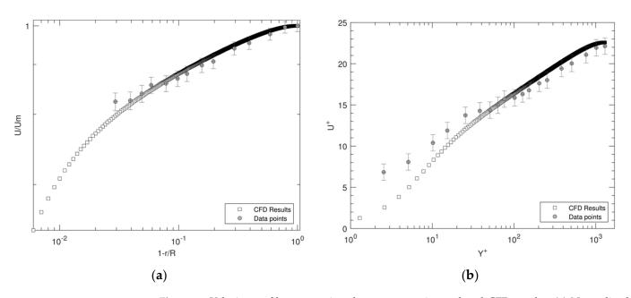
**Figure 8.** Velocity profiles comparison between experimental and CFD results: (a) Normalized velocity versus the dimensionless distance from the pipe wall on logarithmic axes; (b) Dimensionless velocity  $U^+$  versus the dimensionless distance from the pipe wall  $Y^+$ .
