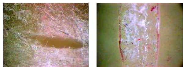
Figure 15. Pictures of air bubbles entrapped in specimens.
