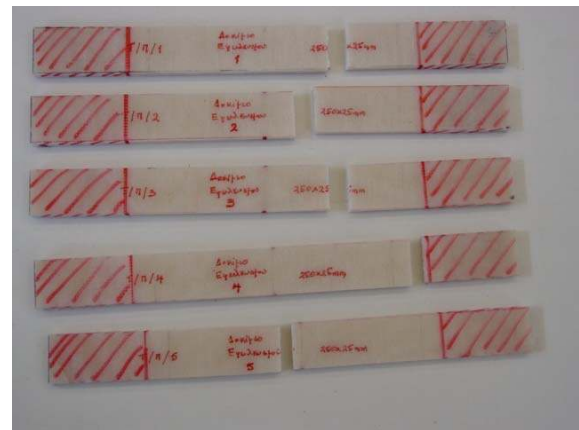
Figure 8. Failure mode of plate coupons in tension.
