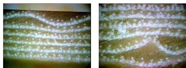
Figure 16. Local misalignment of cotton textile layers.
