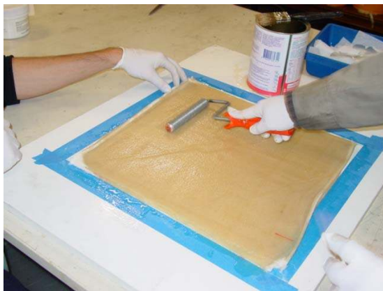
Figure 4. Plate specimen preparation.
