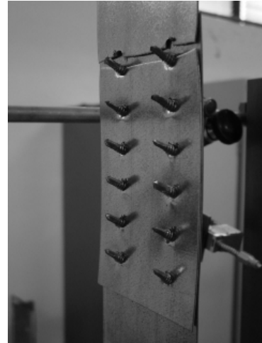
Fig. 4. Thickness of the straps. Fig. 5. Tilting+Pull out. Specimen: 1-1-6,3-4-S350. Fig. 6. Tilting+Net section failure. Specimen: 1-1-6,3-6-S350.
