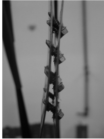
Fig. 4. Thickness of the straps. Fig. 5. Tilting+Pull out. Specimen: 1-1-6,3-4-S350. Fig. 6. Tilting+Net section failure. Specimen: 1-1-6,3-6-S350.
