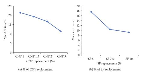
FIGURE 4: Variation of vee-bee consistometer.
