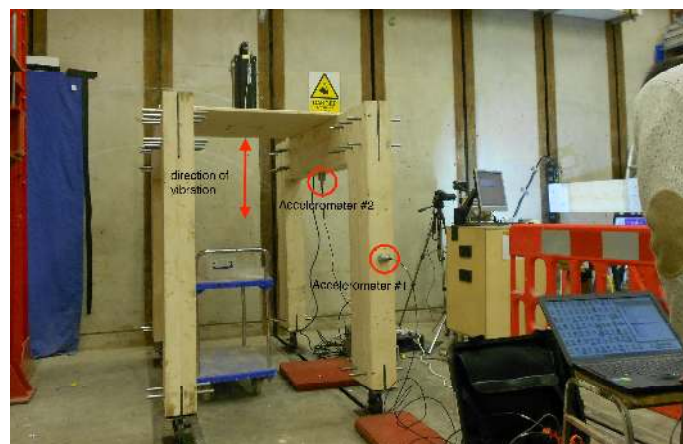
Figure 8. Portal frame under vibration test.
